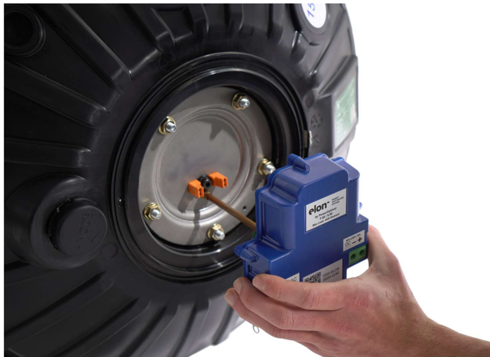
Figure 4.1. STEP 4: Insert the Elon Smart Thermostat stem at least 1/3 rd of the way into the thermostat pocket. Don't insert it fully yet.
