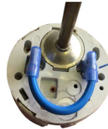
Figure 4.4 Bridging wire fitted to TSE Thermostat
