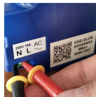
Fig 1 Checking DC voltage Fig 2 Checking AC voltage
