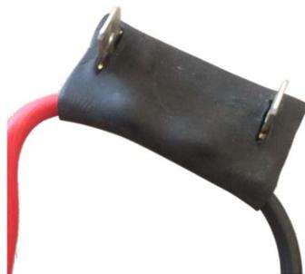
**Figure 4.5** Element connector
