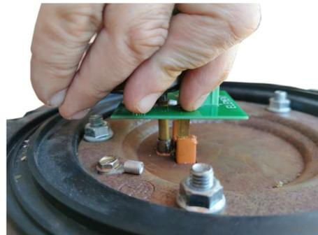
**Figure 4.8 Thermostat & element adapter plugged into element**
