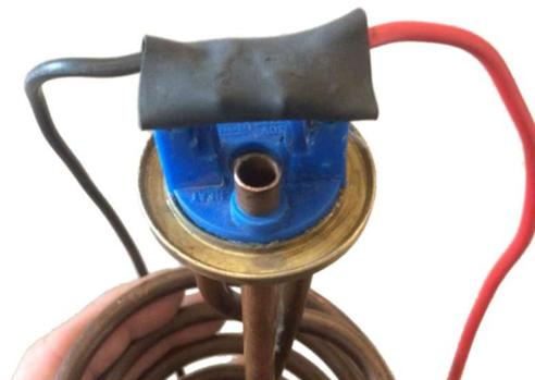
**Figure 4.6** Element connector fitted to flange-type element
