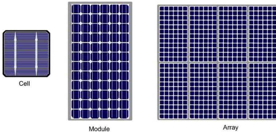
Solar power is generated by solar **cells**, which are arranged in framed **modules**, typically of 60 or 72 cells each. The total set of solar PV modules installed is referred to as a solar PV **array**<sup>4</sup>.
