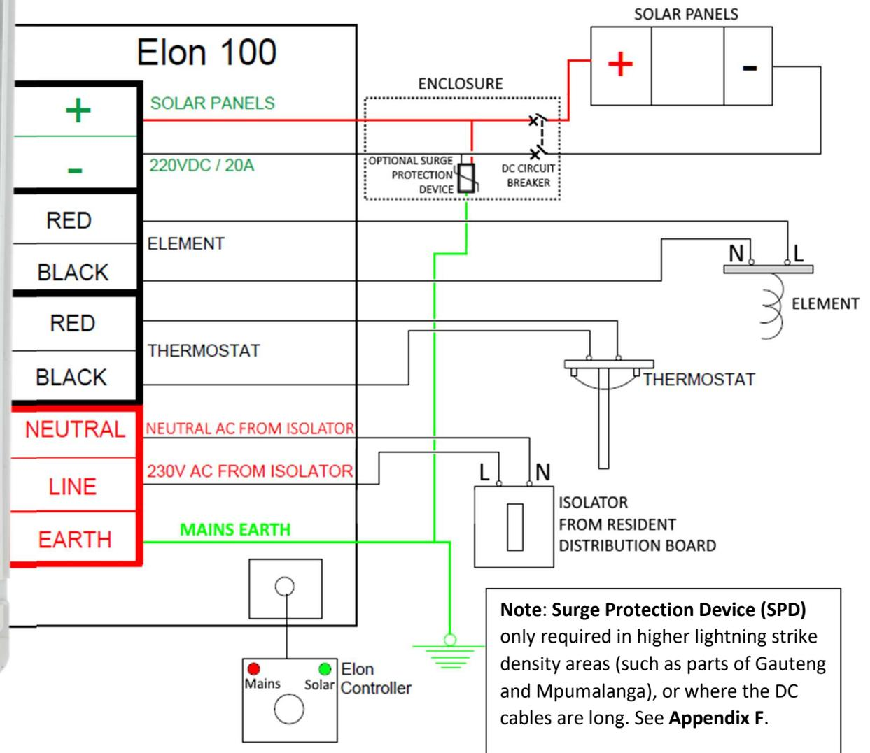
**Wiring detail: Elon 100 with element adapter**
