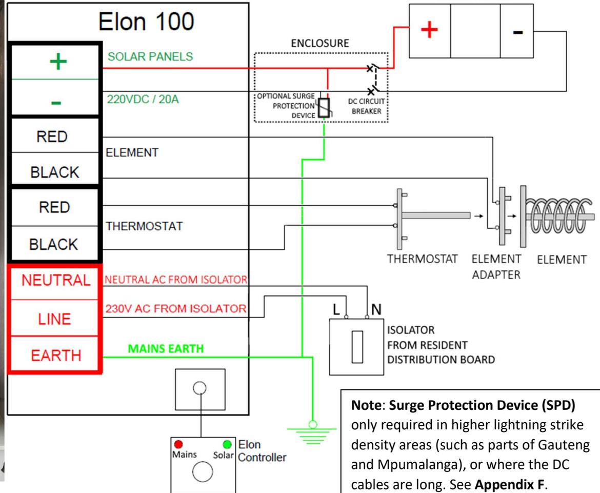
**Note: Surge Protection Device (SPD)** only required in higher lightning strike density areas (such as parts of Gauteng and Mpumalanga), or where the DC cables are long. See **Appendix F**.
