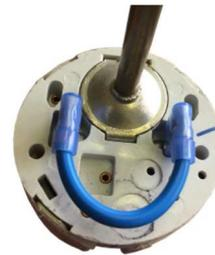
**Figure 4.4** Bridging wire fitted to TSE Thermostat
