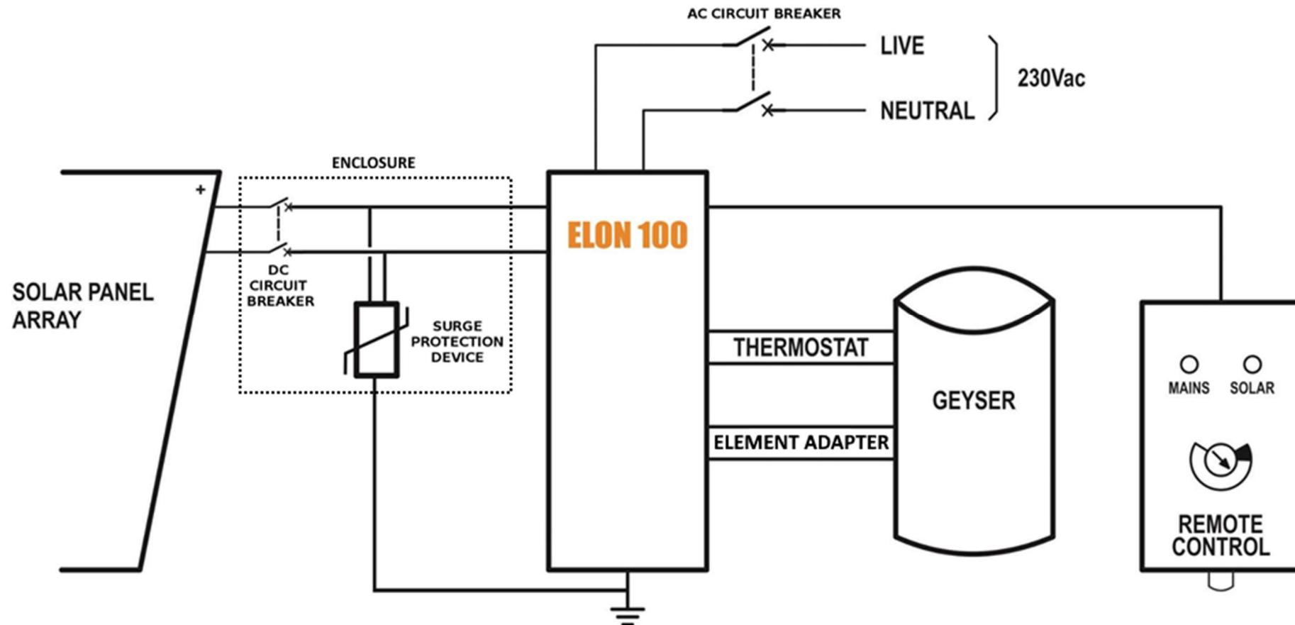
**Note 1:** Both AC & DC circuit breakers or isolators must be installed **within 1.5m of the geyser** (water heater), line of sight.
