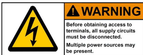
c. Warning – disconnect supply circuits label
