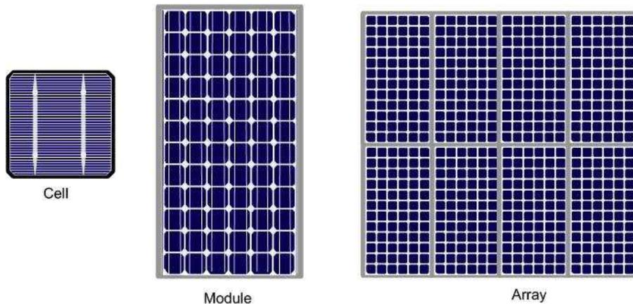
Solar power is generated by solar **cells**, which are arranged in framed **modules**, typically of 60, 72, 120, 144 or 156 cells each. The total set of solar PV modules installed is referred to as a solar PV **array**<sup>6</sup>.
