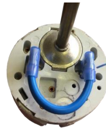
Figure 4.4 Bridging wire fitted to TSE Thermostat
